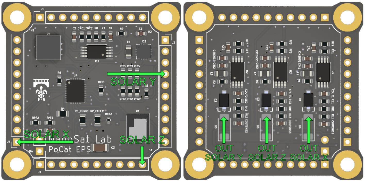
Then to test EPS with the battery, it's important to connect the battery in the correct location. We must not connect the battery negative to the GND, as they are not the same. The battery negative should go to the BATT-. The output of the EPS is the 3.3V output that will be seen by the other SSVs
