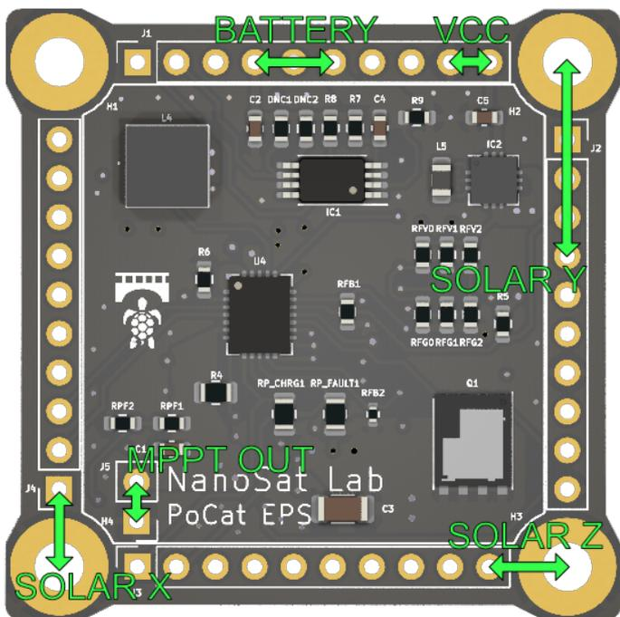
If we encounter a short circuit during any of these checks, we should search for and repair the issue. To do this, we will return to step EPS\_reqBST00 and attempt to resolve the short circuit. Pay attention to any potential tin bubbles that may have remained between the pins of the ICs
