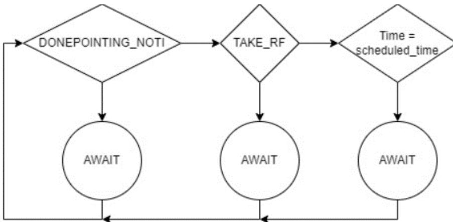
As it can be seen above, the first thing to do in order to get the payload running properly is to check if the conditions required by the Ground Station user are met, this includes three things:
