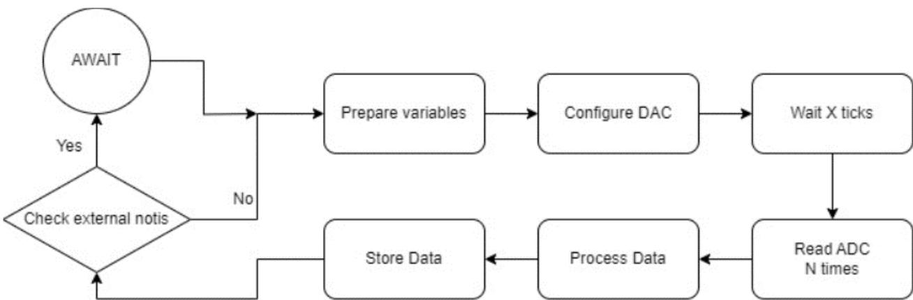
This loop is run as many times as needed in order to scan all the frequency bins forming the L or Ka bands. This scans are slow, so not to block the whole satellite system, every time a frequency bin is scanned the thread checks for notifications coming from the rest of the PQ to pause itself if necessary. Then, once the satellite does not need to have the RFI thread stop anymore, the RFI thread continues from where it was.
