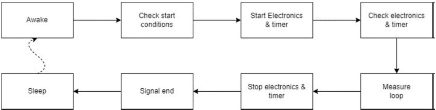
This figure, as stated above, defines how the payload code is structured and its sequential steps. Note that the discontinuous arrow indicates that once the loop has finished, the payload thread enters a sleep mode, waiting for the OBC to awaken him again to restart the loop. So, the first to take a deeper look into is going to be the Check start conditions block:
