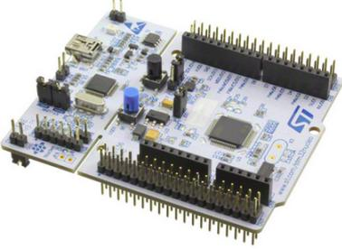
A photograph of the STM32 Nucleo-L476RG board, a blue PCB with a white microcontroller chip, various passive components, and a USB connector. The board is shown from a top-down perspective.                                                            |
