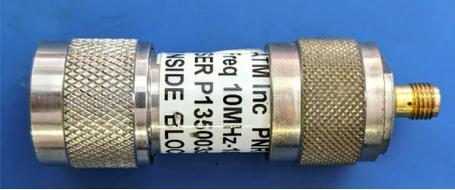
A cylindrical metal adapter with a silver finish. It has an N-type connector on one end and an SMA connector on the other. The text on the adapter includes "ATM Inc. P/N", "SER P-131003", "REQ 10M-Hz", and "INSIDE 5100".                                                                                                                                     |
