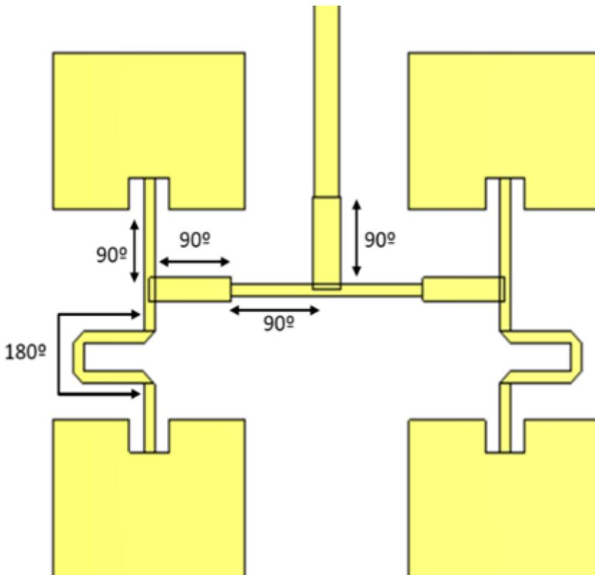
By adding an extra 180° length to access the patches from the bottom of the structure, the waves from the two resonant elements are adding up to each other. In addition, the corner mitering technique has been used as well.
