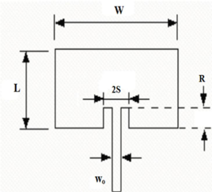
The longitude of the inset R can be calculated with the following equation where  $Z_{in}(R)$  is the matching impedance and  $Z_{in}(0)$  is the impedance at the edge of the patch (if the patch was fed in the end).
