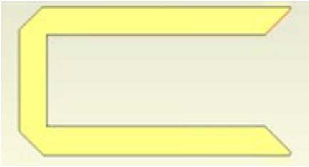
A 90° bend in a transmission line adds a small amount of capacitance to the transmission line, which causes a mismatch. A mitred bend as shown in the previous figure reduces some of that capacitance, restoring the line back to its original characteristic impedance. On the other hand, the whole structure impedance matching is done by two quarter-wave impedance transformers, adjusting the trace's width to obtain the desired characteristic impedance that sets 50 Ω at the output of the network.
