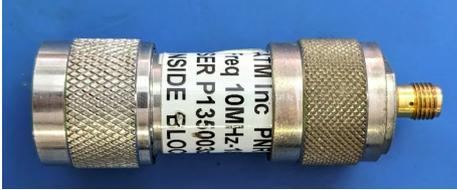
A cylindrical metal adapter with a silver finish. It has an N-type connector on one end and an SMA connector on the other. The text on the adapter includes "ATM Inc. P/N", "SER P-131003", and "SIDE 6100".                                                           |
