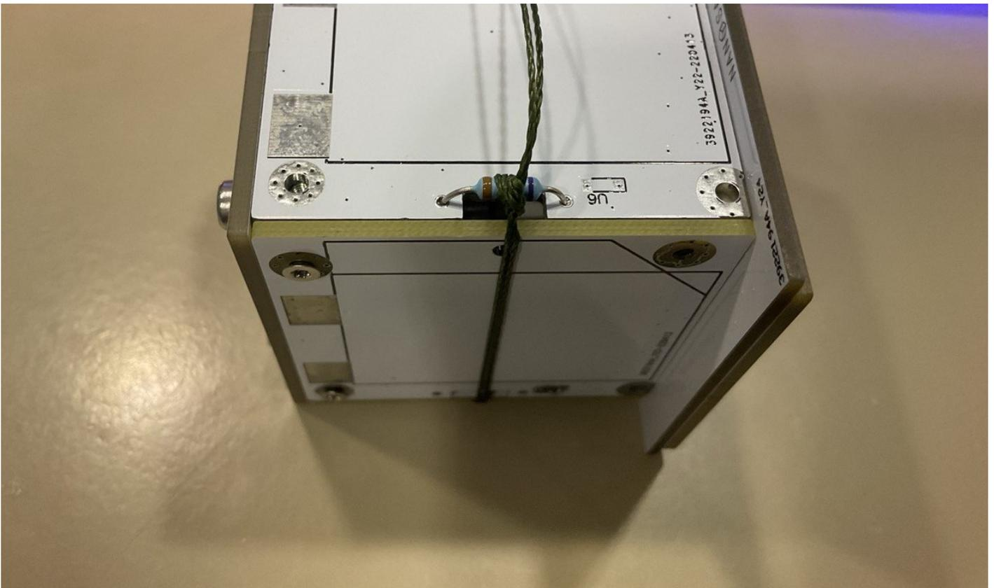
Doing step 1 of the "Antenna Knot" (3) folding in half (instead of just leaving 5cm) results in greater robustness of our knot but increases the melting time of the dyneema to 31 seconds using 3.3V and 450mA.
