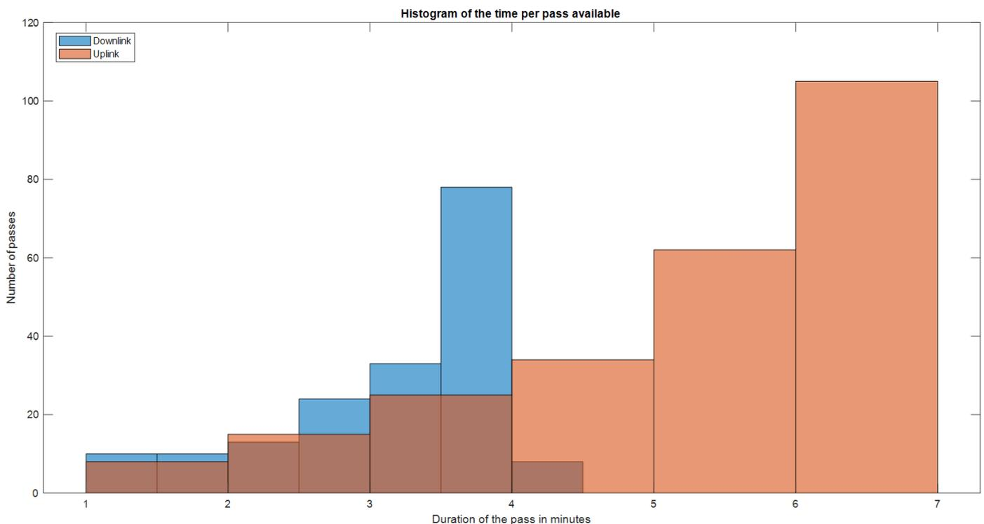
After obtaining the results from Figure G.5, we can compute the data that can be sent during each pass based on the findings presented in [1]. On average, we have 2.49 uplink passes per day over a period of 100 days. For the downlink, we achieve about 1.63 passes per day. Table below
