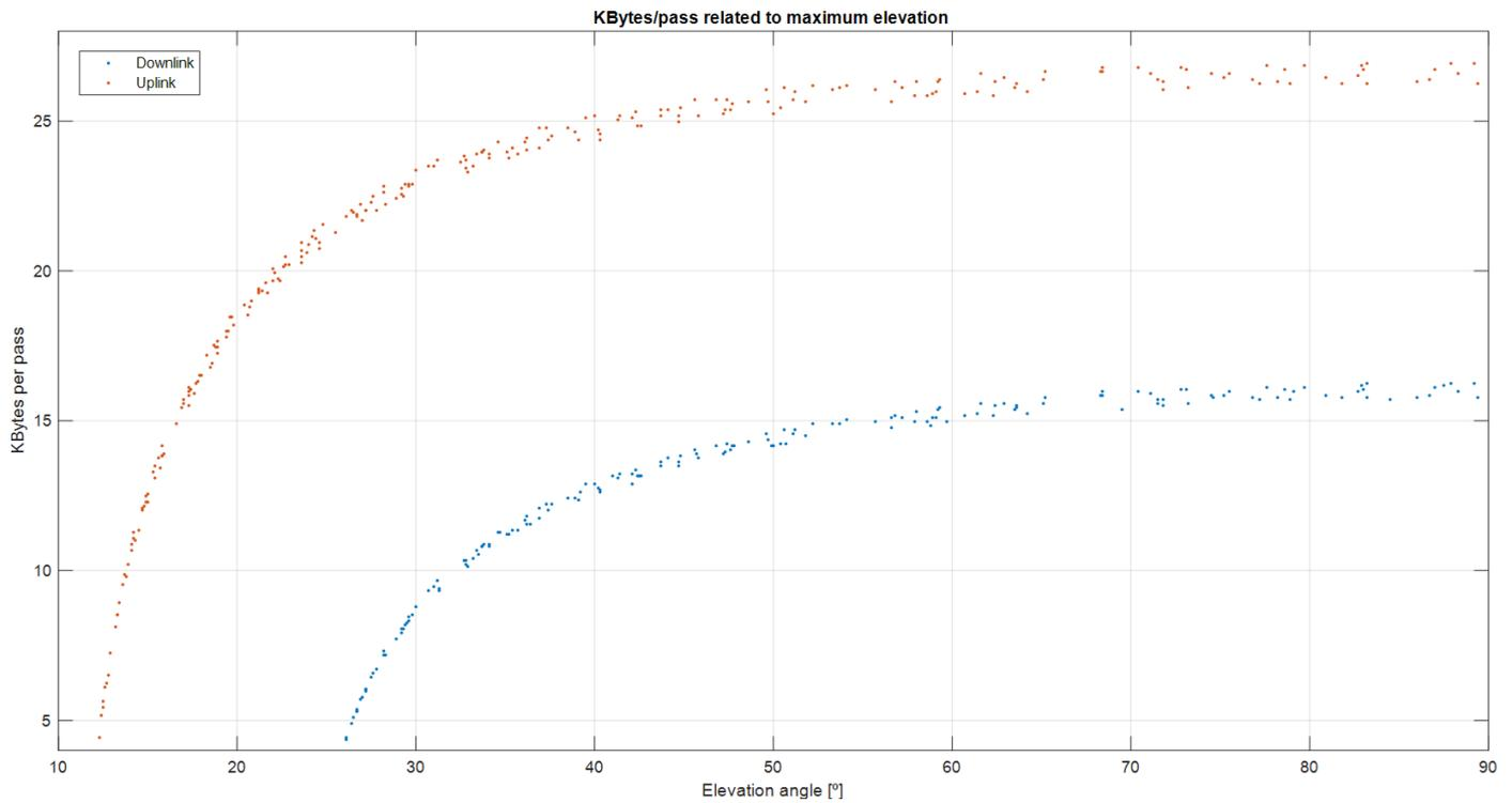
Analyzing the results, we find that the uplink transmission capacity is 20.69 kBytes. For the downlink case, the transmission capacity is 12.52 kBytes, while the L-band payload (which is the payload generating more data) requires 2831 Bytes (2.76 kBytes) to be downloaded from the satellite to the ground station. Therefore, we can conclude that the data budget capabilities are sufficient and that additional stored data could also be transmitted from the satellite to the ground station.
